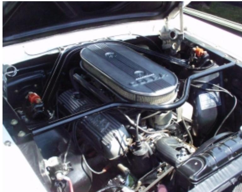
An over-the-counter Carter 8V Cobra set-up lurks beneath that oval Cobra air cleaner
